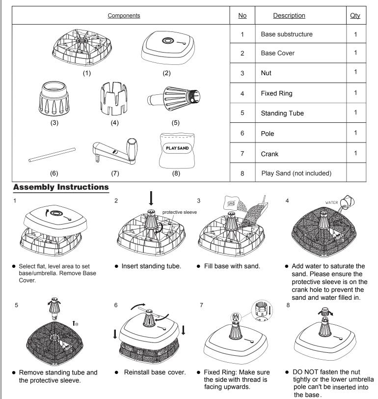
Please note: Make sure to fully fill the inside of the base substructure. If the base is not fully filled, the base cover could be damaged when weight applies to the base cover.
