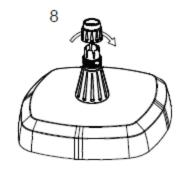
DO NOT fasten the nut tightly or the lower umbrella pole can't be inserted into the base.
