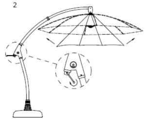
Once the umbrella is fully opened, do not continue to turn crank, otherwise the stopping mechanism will not function properly.
