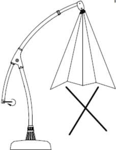
• Caution: Do not open the umbrella before the sliding tube is fully extended. Otherwise the parts will be damaged.
