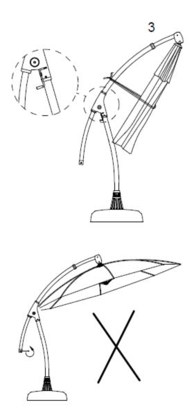
• Caution: Do not close the canopy before the sliding tube is fully extended. Otherwise the umbrella parts will not function properly.
