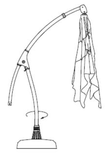
• Release the nut by turning counter-clockwise.
