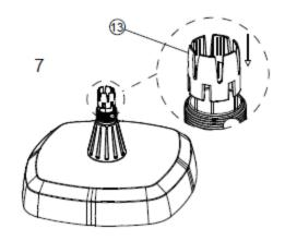
• Fixed Ring: Make sure the side with thread is facing upwards.
