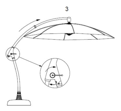
Turn the crank counter-clockwise to tilt the umbrella to desired position when it is fully opened.
