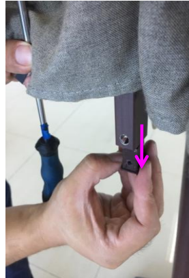
2. Pull out the plug in the long rib.
