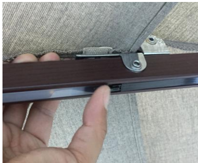
4. Separate the connector of the LED strip from the buckle, then pull out the LED strip.
