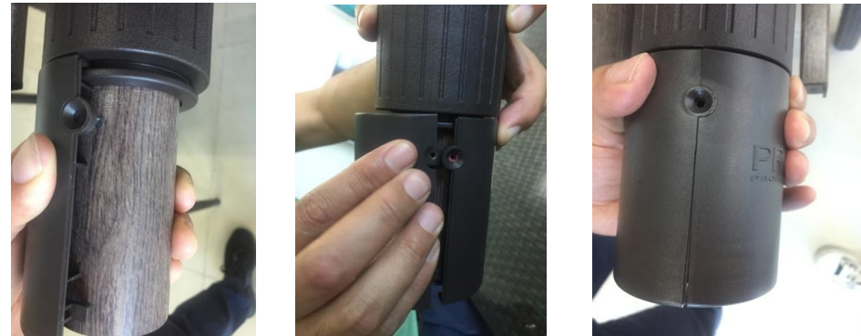
4. Align the screw holes, fasten the new collar.
