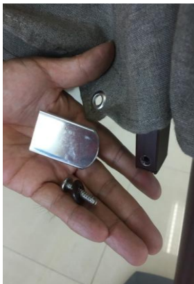
1. Unscrew to remove the rib end.
