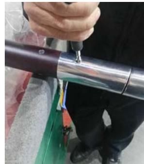
4. Grasp the pole on both end of the tilt mechanism and turn left and right to pull out the lower pole, then remove the tilt from the u
