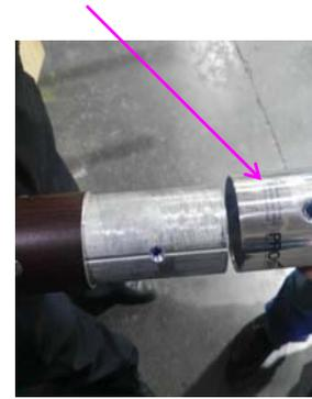
6. Grasp the upper pole and insert the upper of the tilt mechanism
