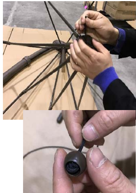
Step 9: Let the new cord go through the lower hub . Make the ribs half open to take out the cord end , go through the stopper then tie a knot and pull into the stopper . Please note the knot is Flemish knot.
