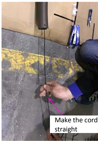
Step 7: Pull the cord at end near lower hub. Make the cord at the other end straight and it will be easier to go through the pole.
