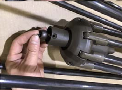
Step 3: Cut off the damaged cord near the low hub. Take out the connector, remove the cap by screw driver and pull out the cord end.
