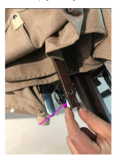
3. Insert the missing black plastic cover into the end of the long rib.
